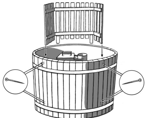
fastened with the supplied screws. The drink holder of the SUB and SIDE is attached to the protective fence.
