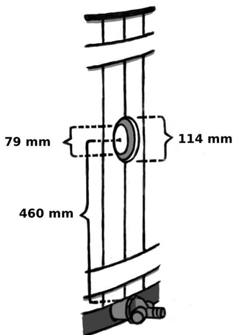
Installation of the Kirami grommet kit for a plastic barrel is very simple, you need to drill a hole just for a single inlet. A Ø79mm hole needs to be drilled into the plastic itself and a >Ø114mm hole into the wood panel at the same level. The hole in the upholstery needs to be bigger in order to tighten the inlet and to have enough space to rotate the components into position.
