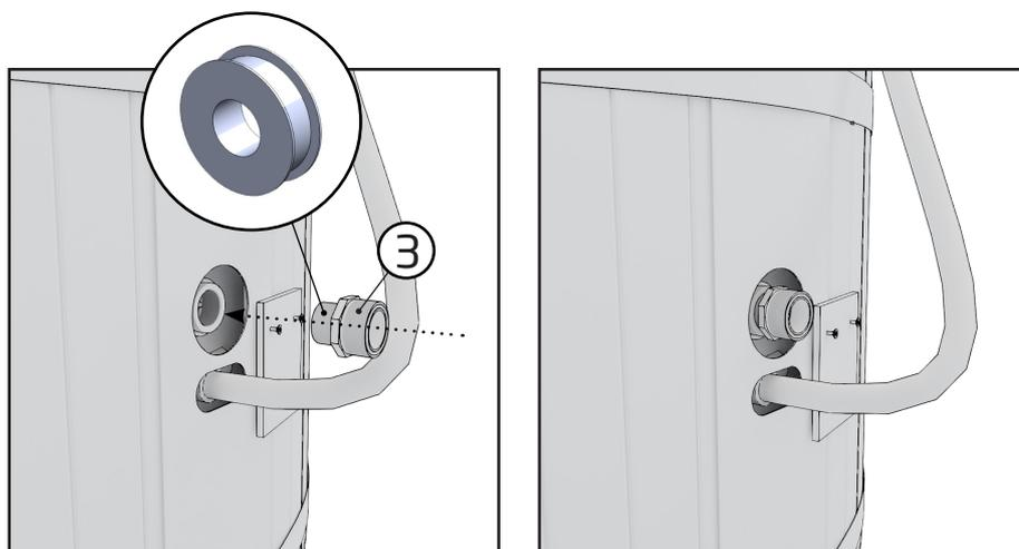
3. Twist the reducer nipple (3) onto the valve on the pool wall. Use pipe tape around the smaller thread, wrapping approximately 15 turns. Do not apply pipe tape to the larger thread.
