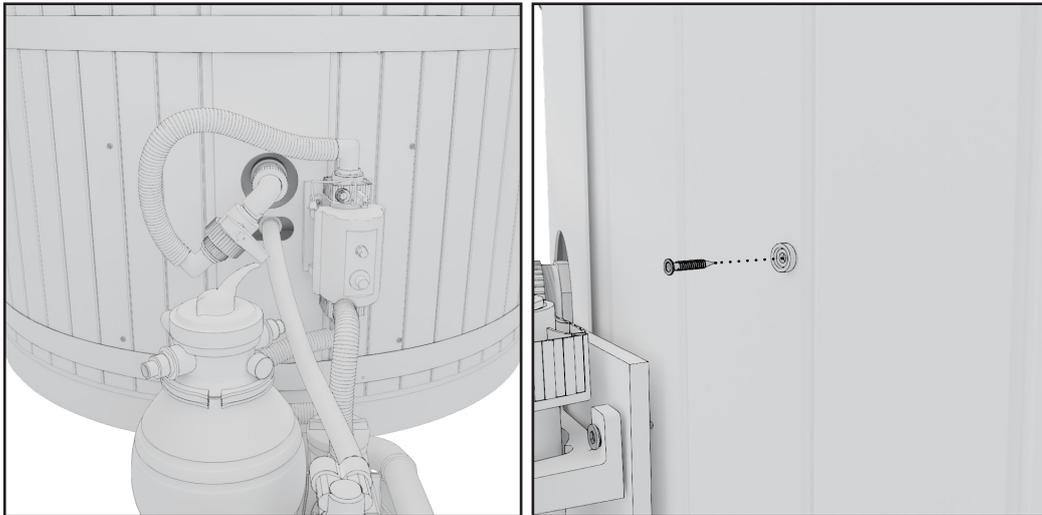
11. Attach the counterparts of the buttons to the paneling with screws at the marked positions.
