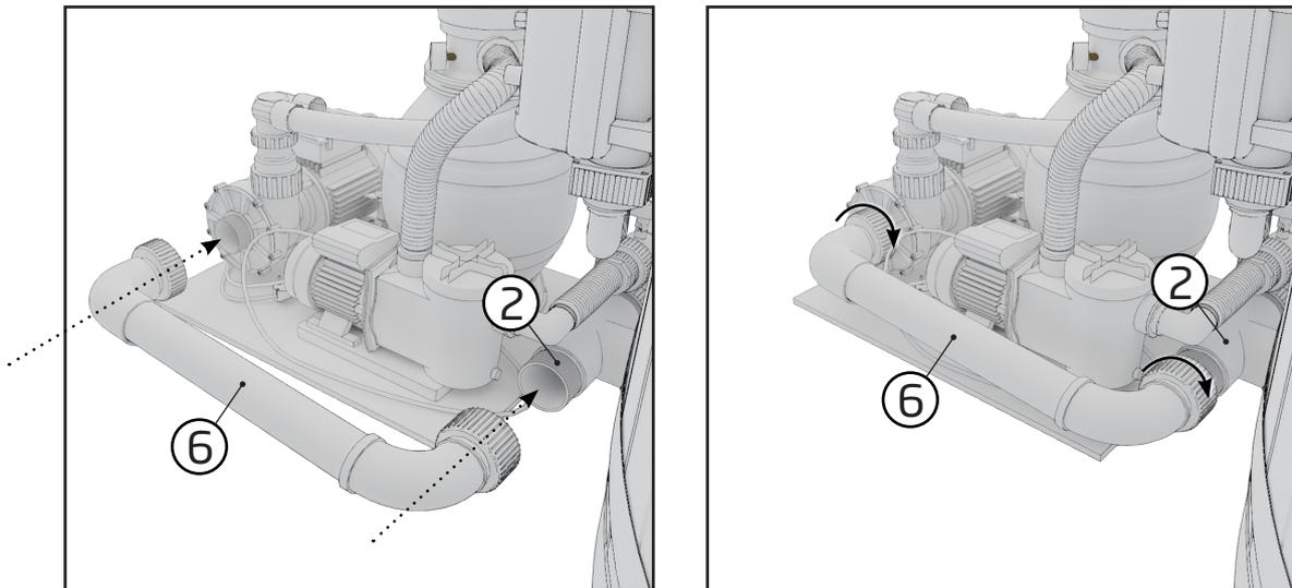
8. Attach the flow system connecting pipe to the T-junction located in the pool and between the system.
