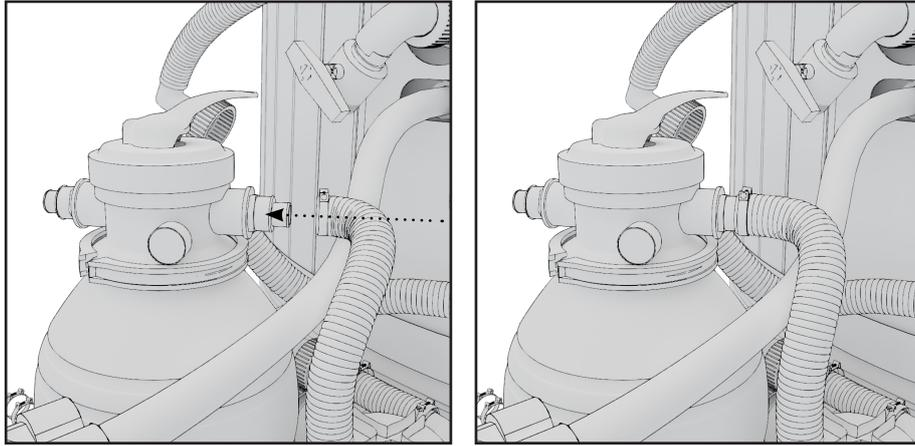
7. Attach the hose from the filter pump to the four-way valve using a hose clamp.
