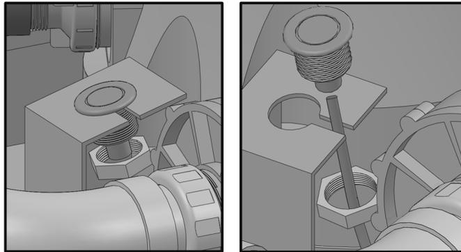
The default location of the start button is on the frame of the flow system. The button can be moved to your desired location. The button is removed by loosening up the nut on the other side. The pipe/hose can also be detached.
