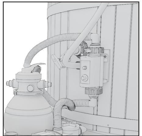
5. Place the main unit next to the hot tub. Ensure that the pressure gauge is positioned as shown in the picture. Turn the 4-way valve if necessary. Lift the heating unit onto the rack on the hot tub wall.
