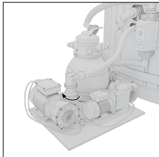
6. Connect the hose that comes from the side of the hot tub to the flow system.
