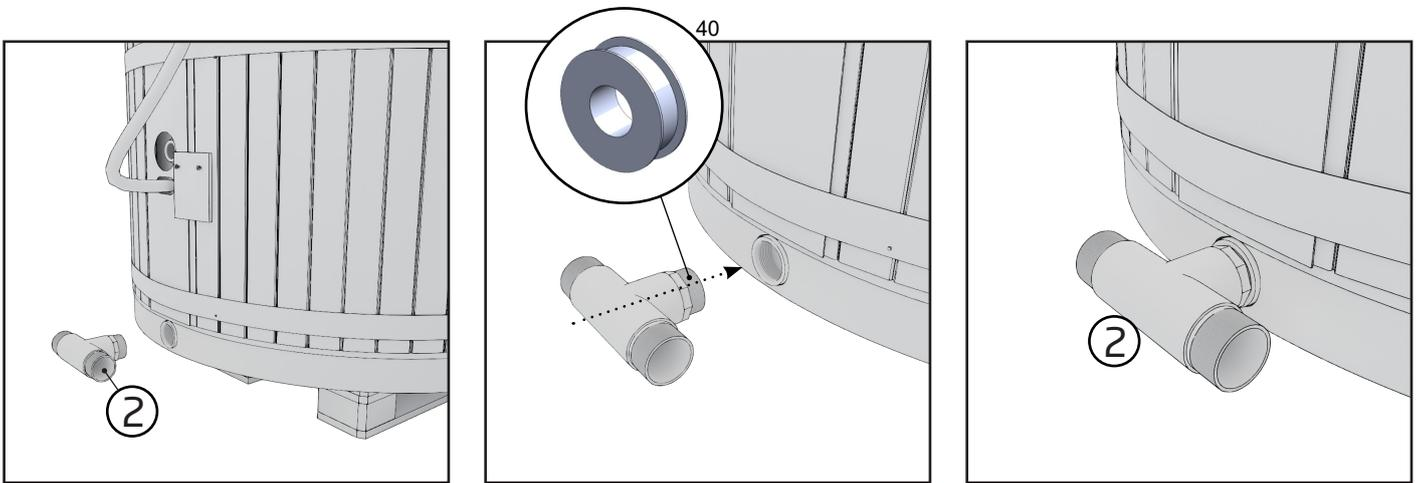
1. Leave the pallet under the tub and screw the T-piece (2.) into the hot tub's outlet. Use plenty of duct tape. Stop turning the T-piece immediately once it is in the horizontal position, because turning it back towards the open position
