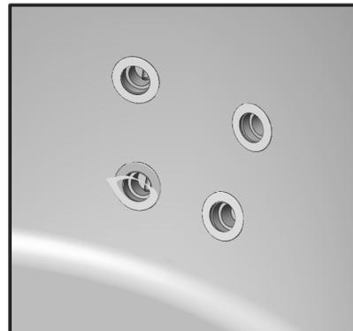
12. To finish, remove the protective plastic from the nozzles inside the pool.
