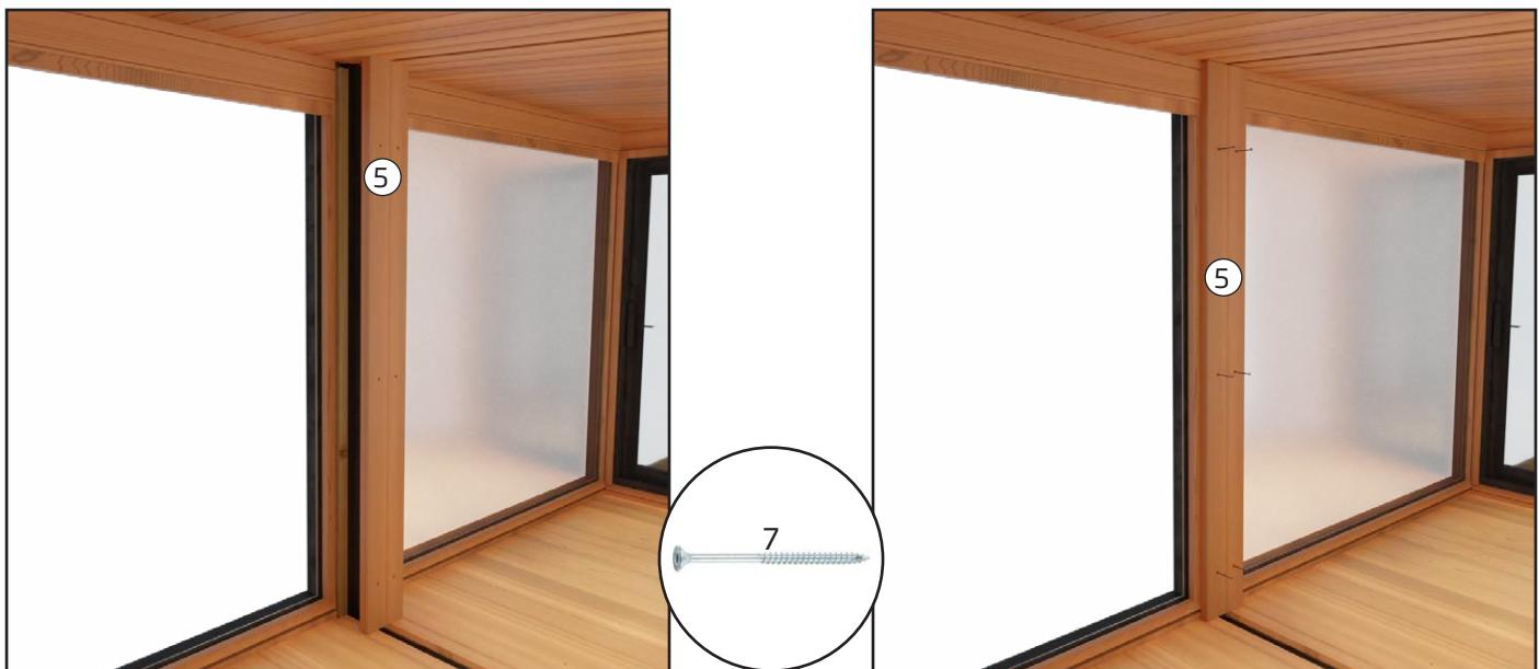
6. Place the strip on the front wall between the modules and fasten with six screws. The strip has pre-drilled holes.
