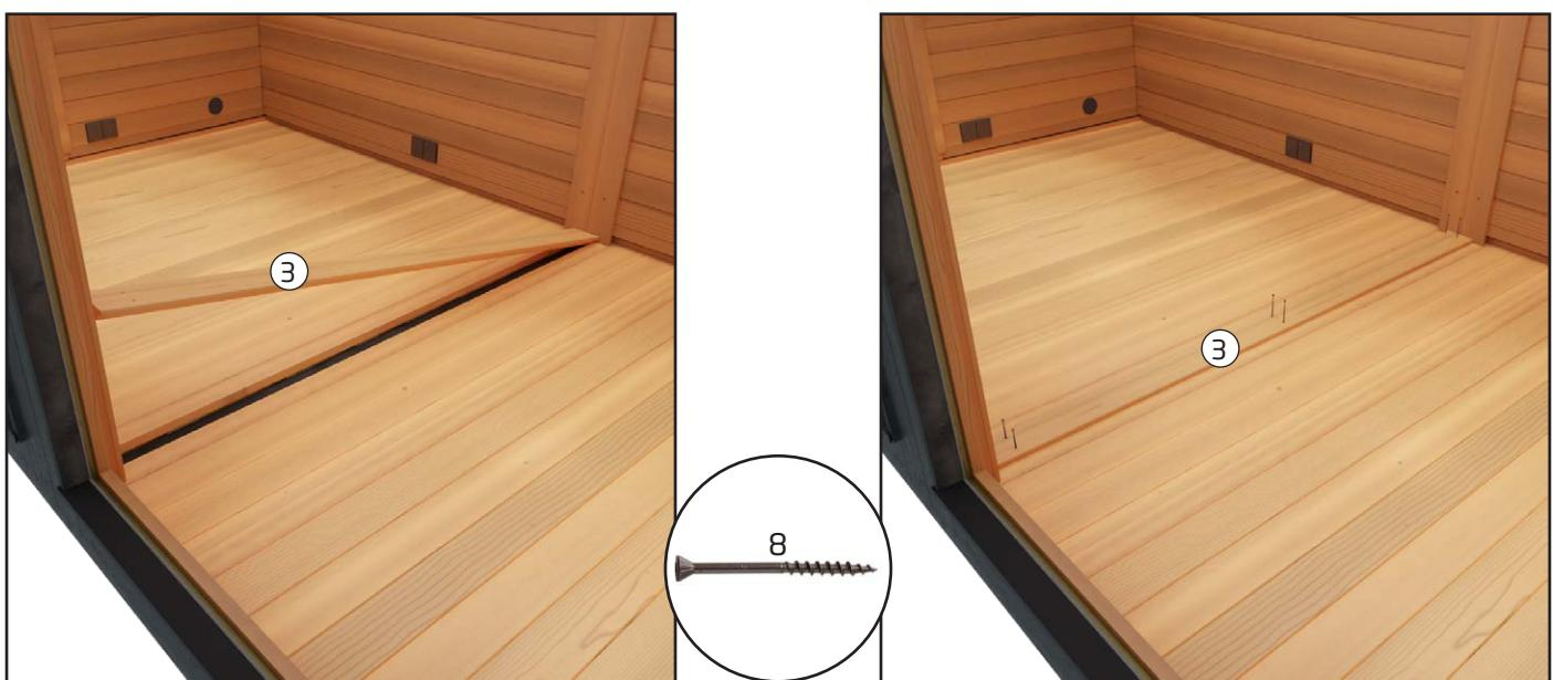
7. Place the cover strip on the floor between the modules and fasten with six screws. The strip has pre-drilled holes.
